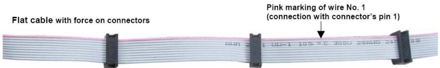
The data line cable when connecting with CBU2 (two connectors) modules:
