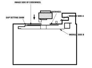
Figure 2. Alignment Tool is Used to Set Height of Codewheel.
