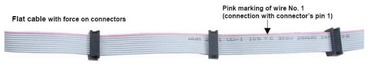
The data line cable when connecting with CBU2 (two connectors) modules:
