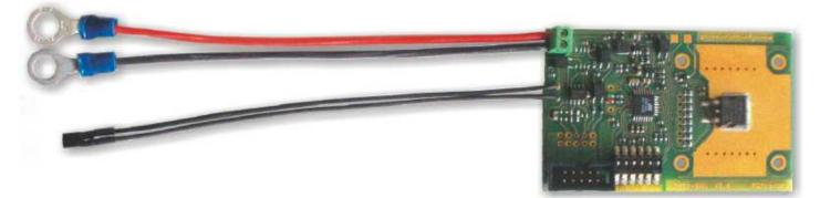
The battery connectors and the battery temperature sensor are provided with each CBU unit.
