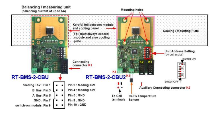
RT-BMS-2-CBU has one data line connector (K1), RT-BMS-2-CBU2 has two data line connectors (K1 and K2). Two connectors allow to connect and disconnect the data line.
