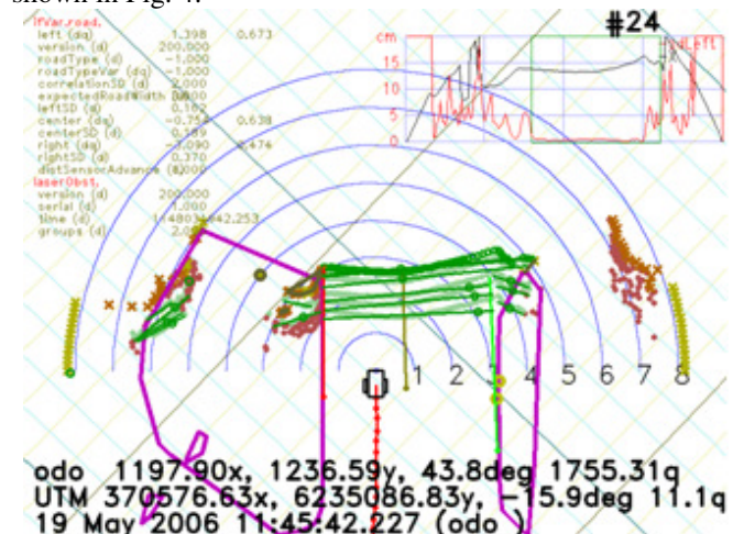
Fig. 4. Operator interface example, illustrating traversable road (green) and obstacles (purple) after treatment of the perception plug-ins.
