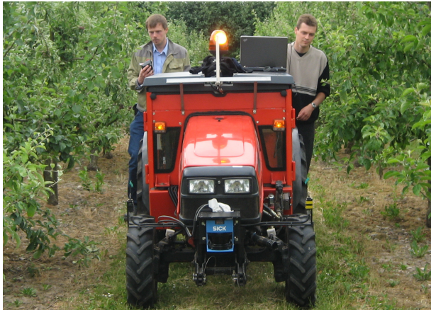
Fig. 5. Autonomous grass cutting between orchard tree rows using topological feature-based localization in tree rows through the MobotWare framework.
