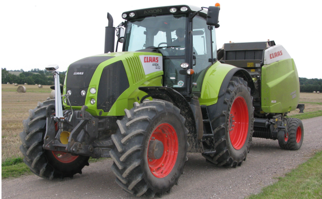
Fig. 6. The Agrocom stereo vision equipped Claas AXION 840 runs MobotWare for autonomous field operations.
