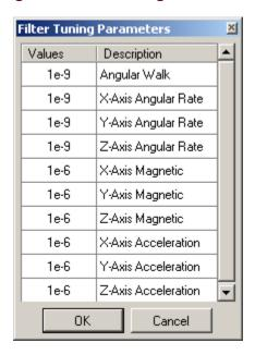
**Figure 2 - Filter Tuning Parameters**
